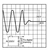
4-(2). DC coil surge voltage waveform (With diode) Diode characteristics: Reverse breakdown voltage: 1,000 V Forward current: 1 A
