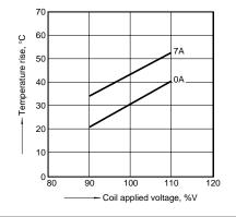
2-(2). Coil temperature rise (2 Form C/DC type) Measured portion: Inside the coil Ambient temperature: 70°C 158°F
