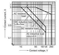
1-(2). Max. switching capacity (4 Form C type)
